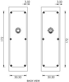
The recess measurement required to fit this item is taken from the back
